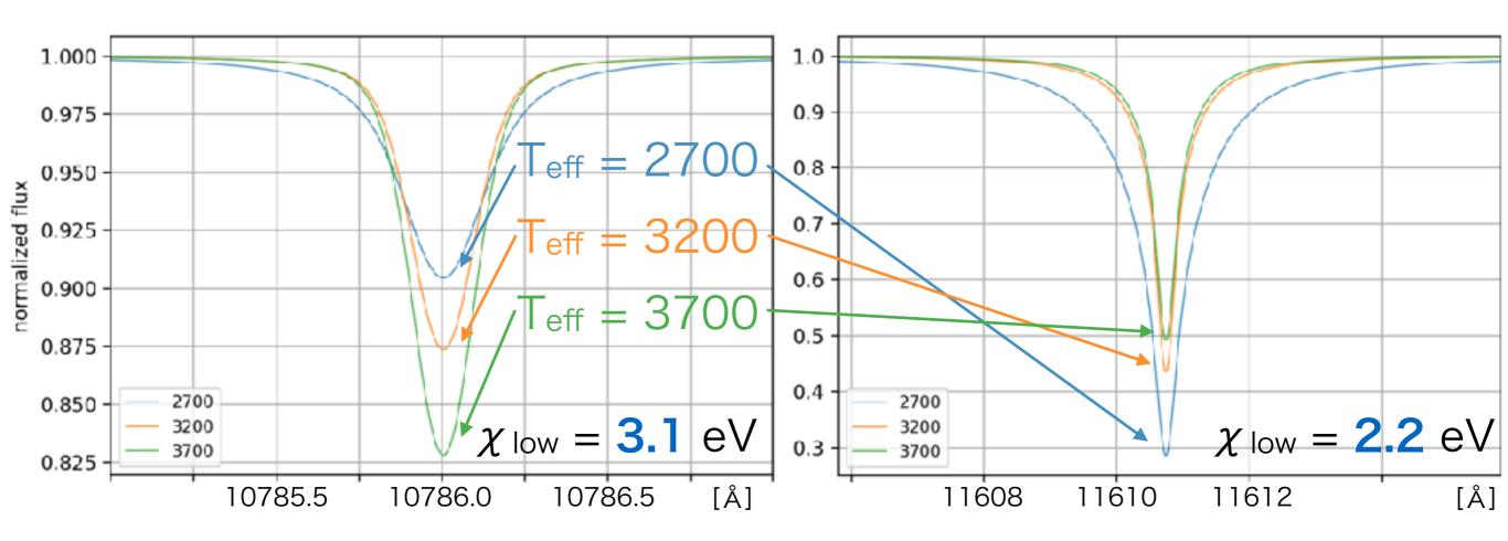
The metallicity-sensitivity of each line is also affected by the **temperature-sensitivity**, which is **specific to each line** (lower excitation potential)
