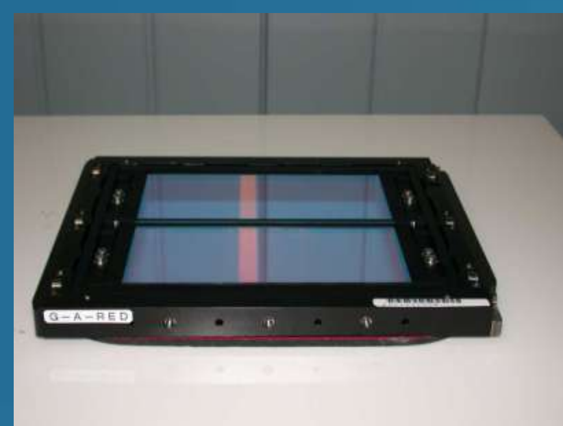
Fig.4 Red grism : Two unit grisms 17.0 cm x 7.4 cm x 1.7 cm x 2 (top and bottom) cover the FOV of Suprime-Cam. This grism frame is inserted in the optical path like a band-pass filter.
